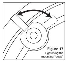
install the speaker, first rotate the dogs inward. Insert the speaker into the cutout and tighten the dogs by turning the screws clockwise. DO NOT OVER-TIGHTEN THESE SCREWS. Over-tightening the clamps may make the grille difficult to install. **(See Figure 17)**.
